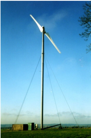
Figure 2b: Two blade horizontal axis turbine
